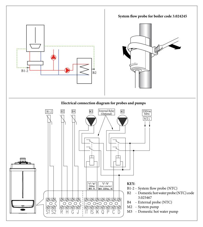
Using the "direct management" system without the cascade regulator, and installing the system flow probe Kit (for direct combination with the boiler) code 3.024245 (optional), it is possible to manage:
