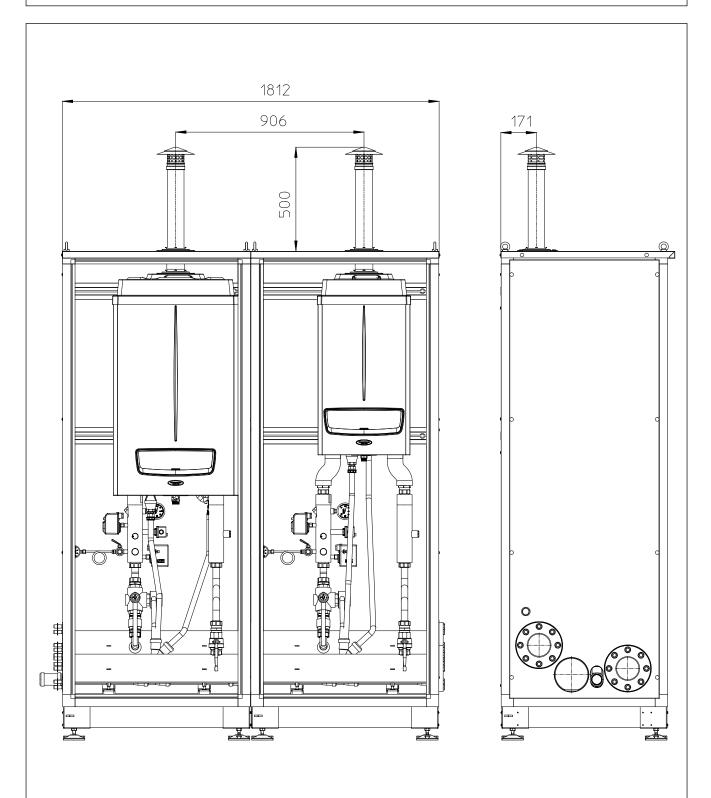
NOTE: Having the flue exhaust separated and a INAIL kit for each generator, you can also make mixed sets with VICTRIX PRO 2 ErP generators having different powers. It is not possible to use flue manifolds for boilers in sets.
