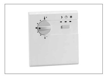
The modulating room thermostats (not traditional On/Off) functions only when coupled wit the cascade regulator and allows regulation of the room temperature of one of the zones into which the plant is divided (both in individual and cascade installation).
