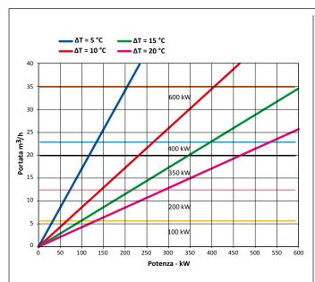
The above graph provides information to enable you to choose the most appropriate separator based on the design data.
