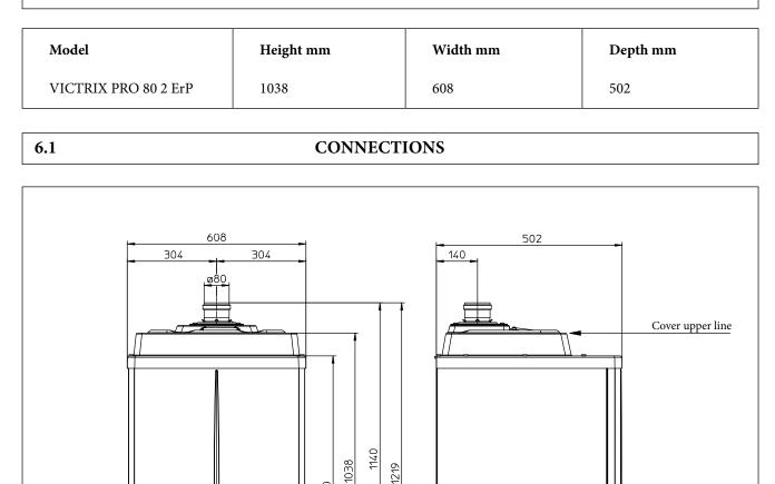
SC = Condensate drain 25 Ø mmDistance between cover upper line and Distance between cover upper line and 80 Ø drain bend axis: 160 mm concentric intake-exhaust bend axis Ø 80/125 190 mm
