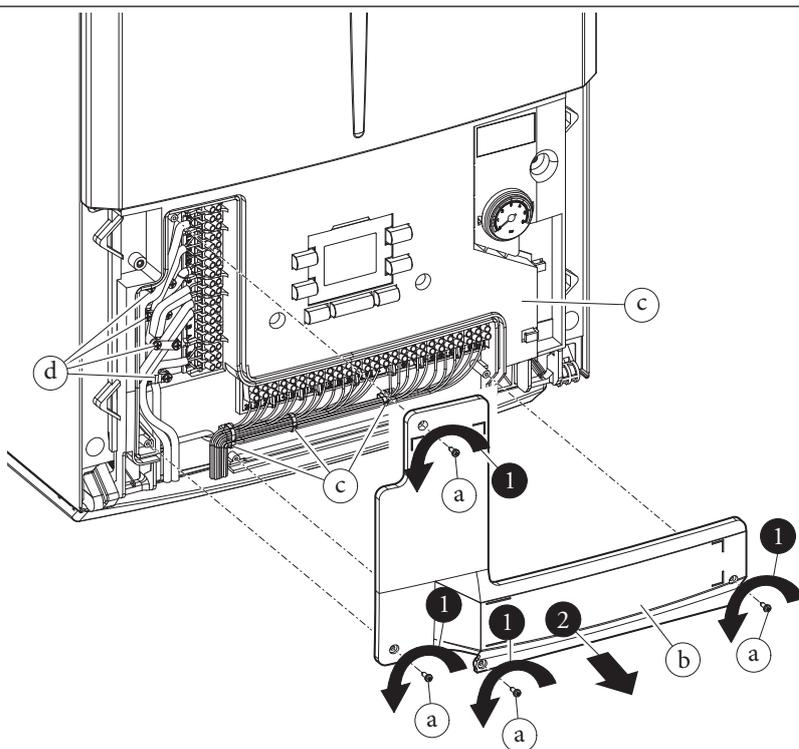
**Vertical terminal block electrical connection diagram.**
