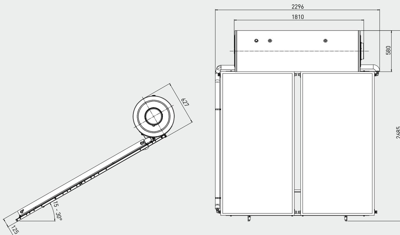
Dimensions refer to on sloped roof installations.
