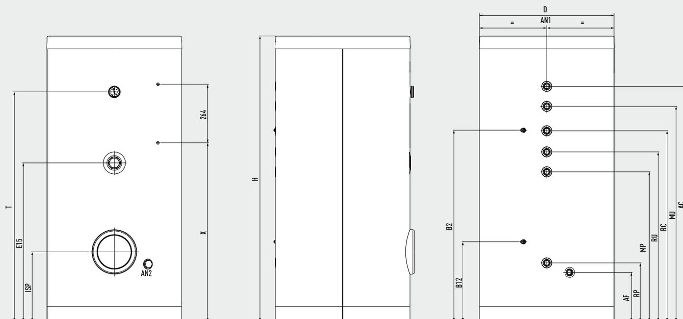
N.B.: while performing the connection, set up a drain fitting and an interception cock at the cold water inlet (AF) to facilitate maintenance operations.
