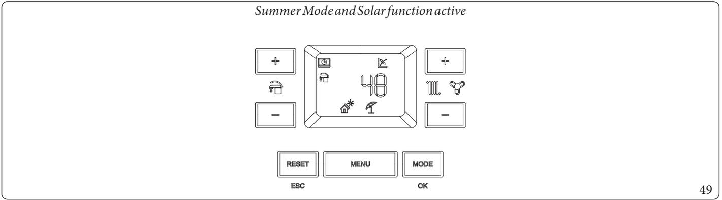
When the water supplied by the solar system is at a temperature lower than what is set, or if the “Solar ignition delay” time has elapsed, the system switches on to bring the DHW to the set temperature. At this point, the solar function symbol will go off.
