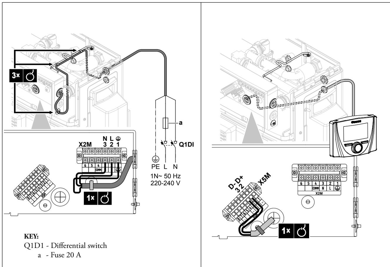
**Features of the outdoor unit connection.** The outdoor unit power cable (not standard supplied) must be suitable for outdoor installation and must have at least a flexible polychloroprene sheath (code IEC:60245 IEC 57 / CENELEC:H05RN-F).
