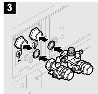
**N.B.:** In addition to the thermostatic antifreeze valve, a vacuum breaker valve is also supplied, which must be installed on the heat pump delivery valve (MHT) by removing the cap present.
